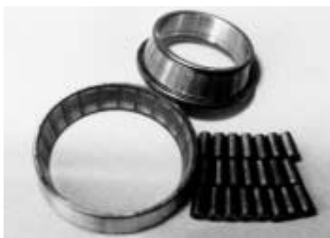
Fig. 15-12 Corrosion on Tapered Roller Bearing
